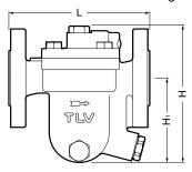
DIN type is shown. ASME type has welded on flanges.
